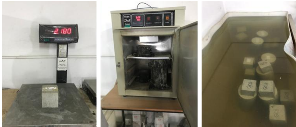
Figure 7. Weighing and drying of geopolymer samples
