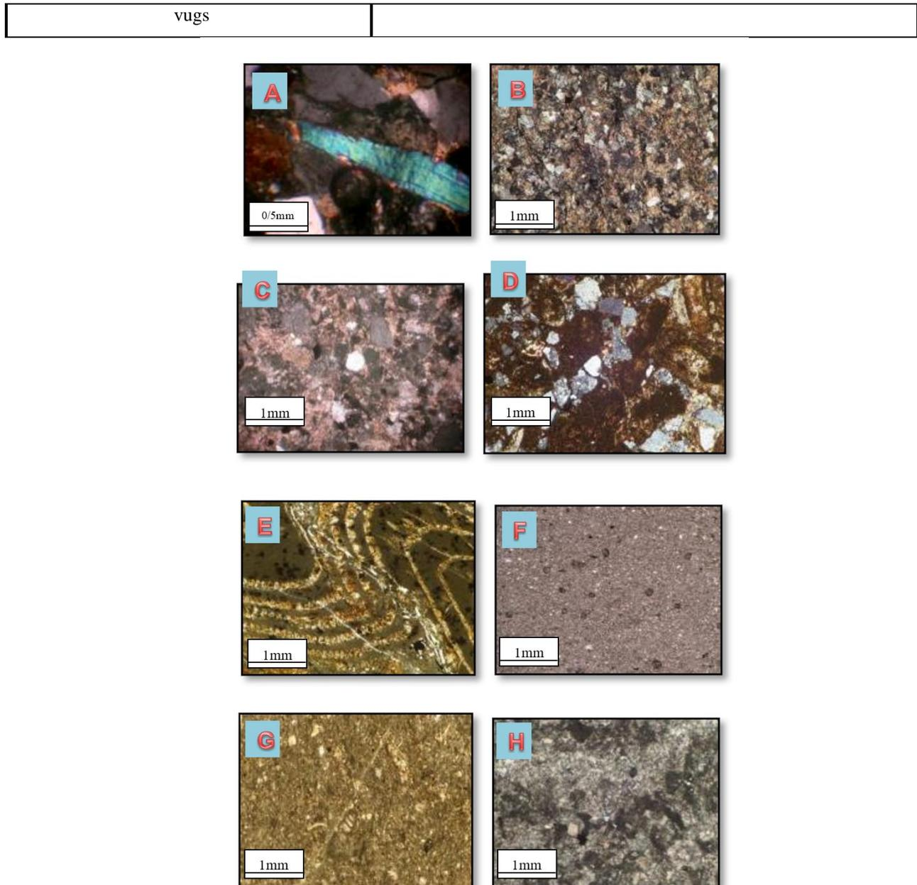
**Figure 10.** A: Bending of mica minerals in sandstone (PPL); B: Carbonate cement in sandstone (PPL); C: Presence of granular calcite cement (PPL); D: Micritized skeletal grain in carbonate rock (PPL); E: Convex-concave contact between *Alveolina* fossil grains (PPL); F: Neomorphism (PPL); G: Biogenic features in carbonate rocks (PPL); H: Dolomitization in carbonate rocks; crystals exhibit shaped to amorphous fabric (XPL)
