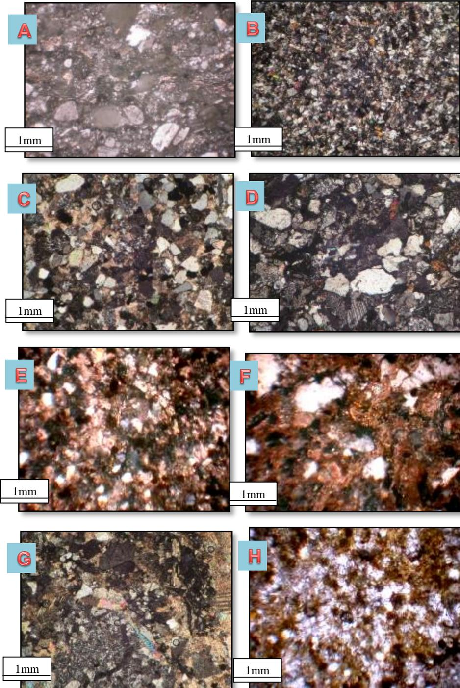
**Figure 7.** A: Arkose petrofacies (PPL); B: Sub-arkose petrofacies (PPL); C: Lithic petrofacies (PPL); D: Sub-lithic petrofacies (PPL); E: Amorphous quartz minerals in the carbonate matrix of lithic sandstone (PPL); F: Petrofacies of calc-litite sandstone (PPL); G: Microconglomerate (PPL); H: Clay minerals in calc-litite sandstone (XPL).
