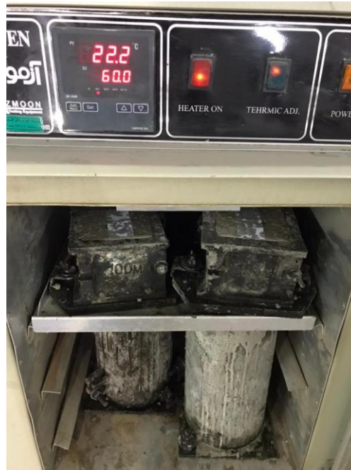
Figure 5. Sample Placement Conditions in the Oven at 60°C
