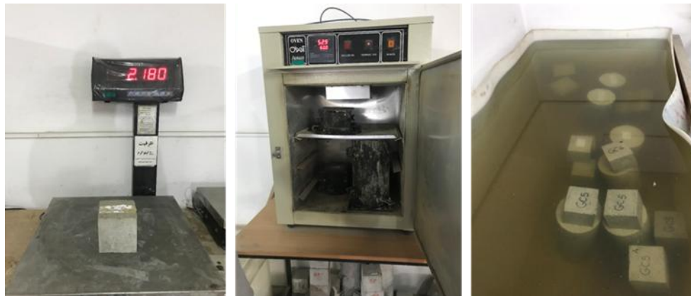
Figure 7. Weighing and drying of geopolymer samples
