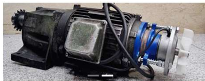
Figure 5. Induction motor equipped with an electromechanical brake
