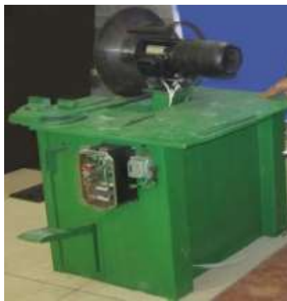
Figure 10. Industrial cutting machine (circular saw) equipped with the intelligent life-protection and amputation-prevention system
