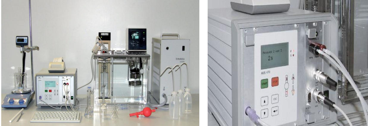
Figure 2. Rotary viscometer (rheometer) with a coaxial cylinder.
